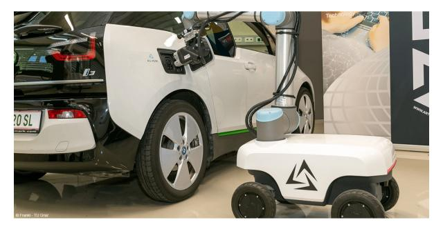
The purpose of the robotic arm is to improve accessibility of charging by reducing the user involvement and streamlining the process. Today, about 22% of the UK population has accessibility needs, which new technologies need to accommodate for. Lowered mobility and wheelchair usage can create barriers in the use of traditional EV charging stations because fast chargers run at very high voltages and are water-cooled, making them very heavy and difficult to manoeuvre.
